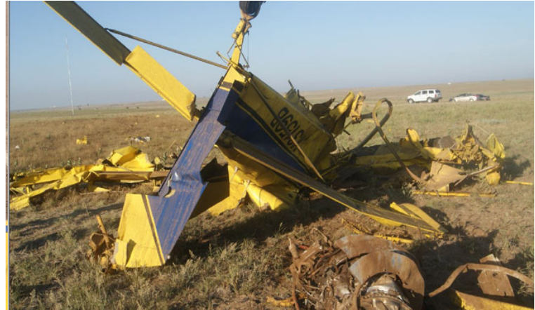
Fatal Air Tractor collision with a meteorological evaluation tower (MET). August 2013.
