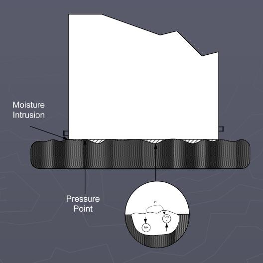
Non-uniform tank base can allow moisture to collect underneath tank
