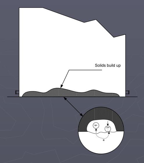
Solids create stagnant voids where accelerated corrosion can take place - pitting
